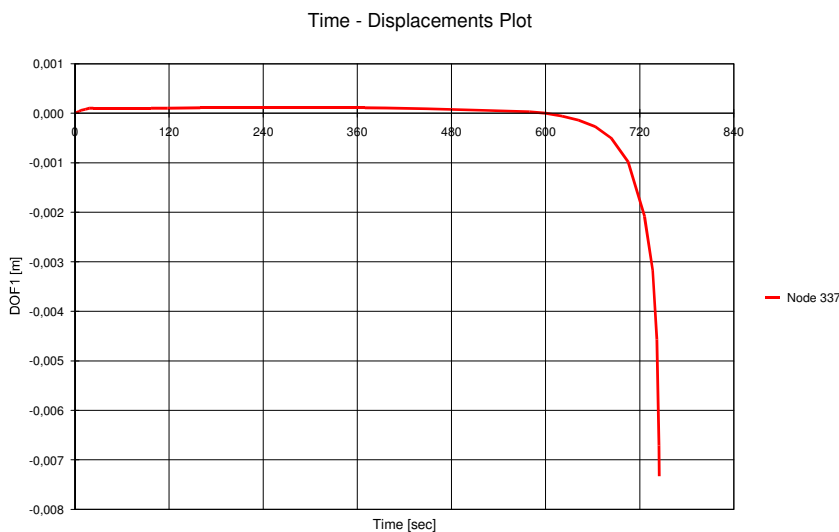
Fig. 6 - Evolution of the lateral displacement in a critical point versus time of exposure to fire
