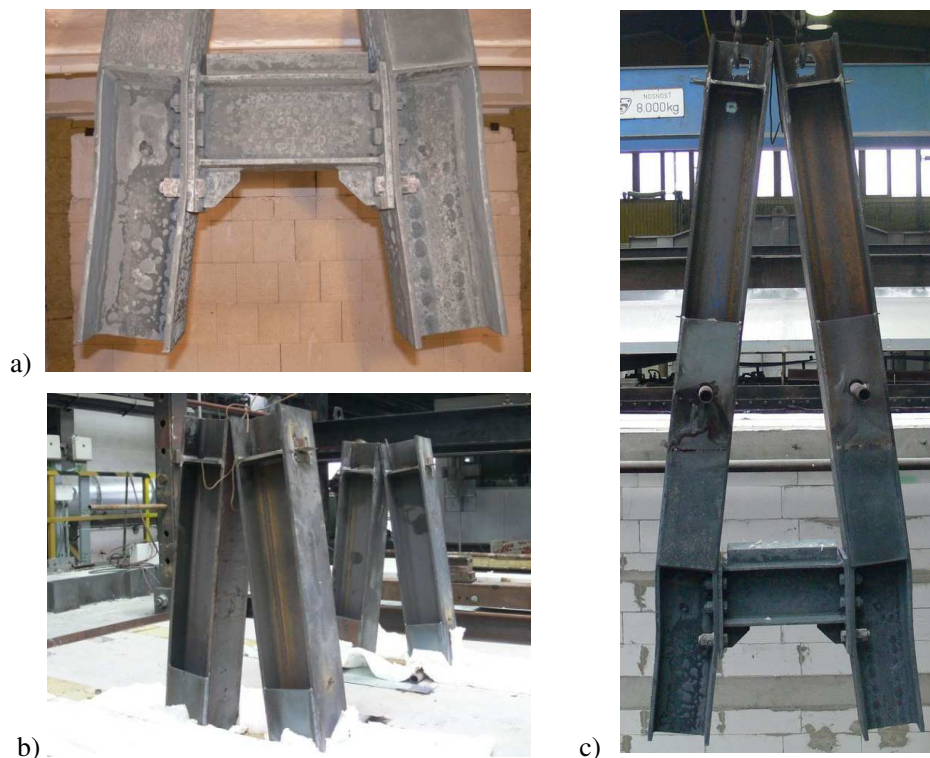
Fig. 6 - Specimens E15 after the test, a) inside the furnace, b) outside the furnace. c) specimen E15 taken out the furnace.
