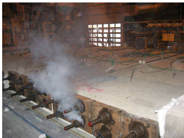
Figure 2. Photo of large test specimens of tunnel concrete during fire testing.
