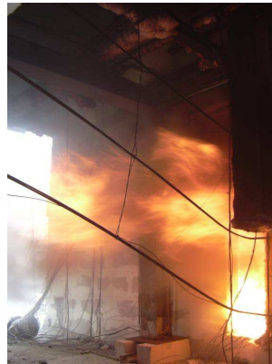
Fig. 1 – Experimental external flaming (Efectis France).
