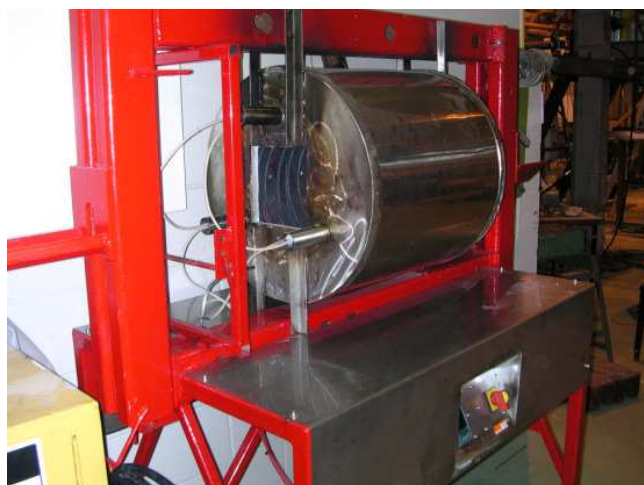
Fig. 2 - The test frame and furnace used for the heated tests and fire testing.
