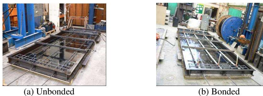
Fig. 1. Moulds used for casting the post-tensioned concrete slabs
