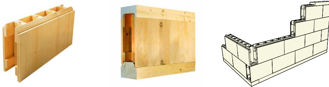
Fig. 1 – STEKO basic hollow timber block made from cross-glued boards (left), timber block with base plate and top plate (center) and schematic timber block wall construction (right).
