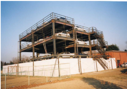
Fig. 1. Large full-scale fire test structure
