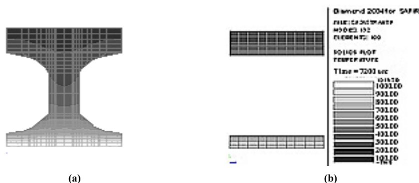
Fig. 2. – Temperature distribution of SP265 Ergon after 2hr. of ISO fire from (a) longitudinal beam (b) transverse beam
