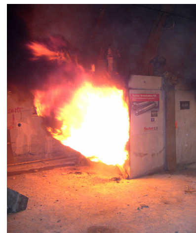
Fig. 8 - The north channel of the Virgolo tunnel covered with six different lining systems and the "mini-tunnel" containing four concrete panels during the hydrocarbon-pool fire test.
