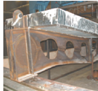
Post web buckling mode failure B1
