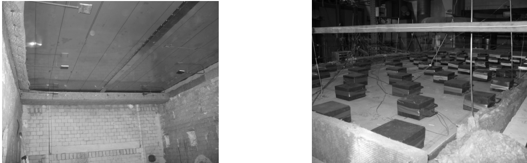
Fig. 3 – Large scale test setup: furnace (left) and applied variable loads (right).
