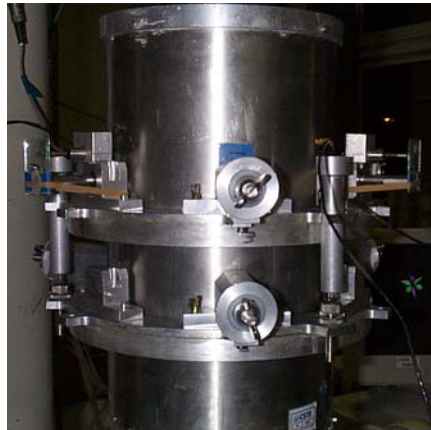
Fig. 2 – Hot mechanical tests apparatus with radial strain measurement.
