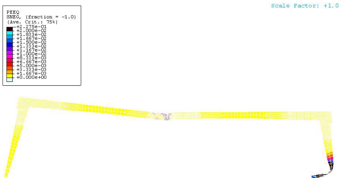
Fig. 8 Local collapse of un-protected column.
