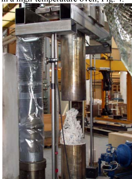
Fig. 4 - Electrical oven with LVDTs and cooling equipment.
