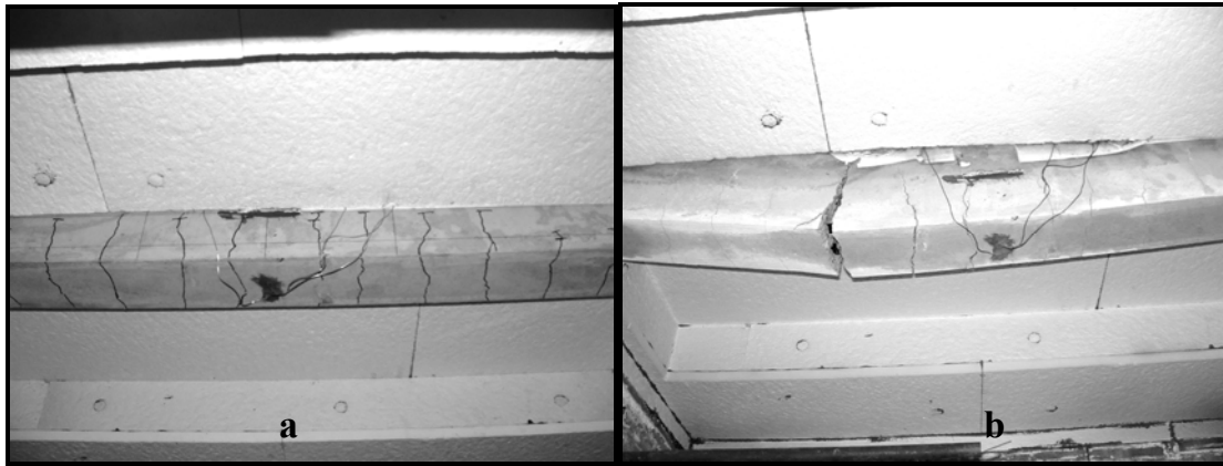
Fig. 4 - CFRP specimen in the furnace before and after testing.
