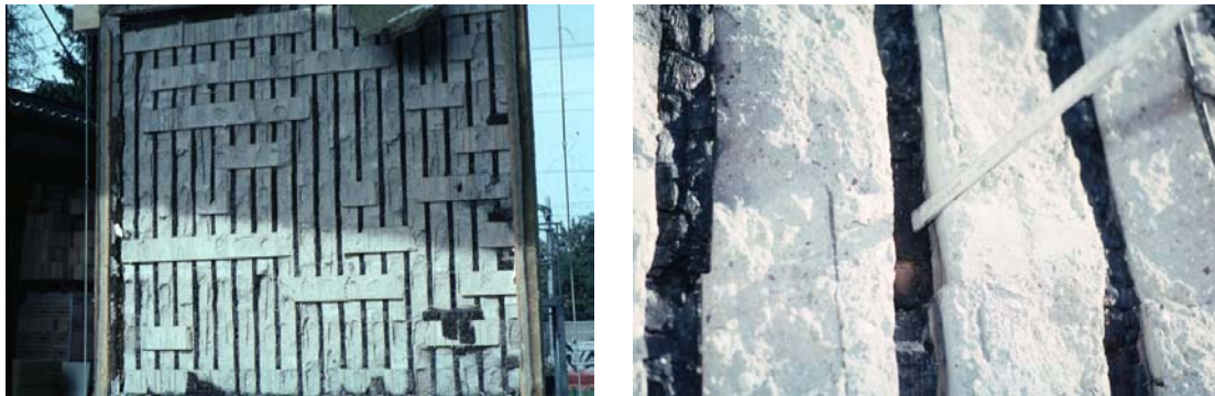
Fig. 13 – Fire exposed side of wall 5 after the fire test (left) and detail of one-dimensional charring of the timber webs between the concrete (right).
