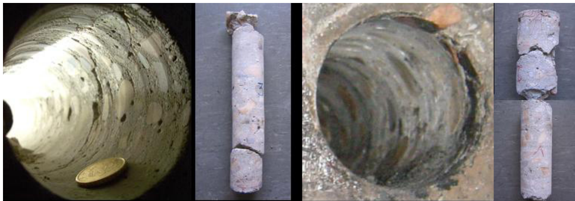
Figure 6. cores and holes taken from column1, left, and column 2 right.
