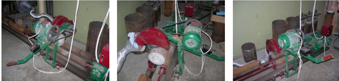
Fig. 2 – Cutting machine used for preparing of the specimens.
