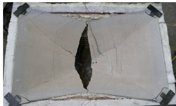
Fig. 4 – Mode of failure for test slabs at elevated temperatures.
