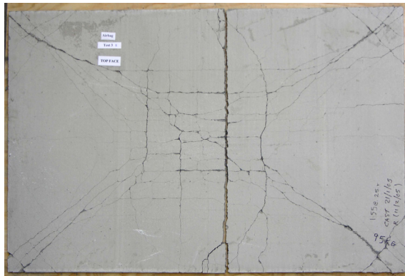
(a) Fracture of reinforcement along short span
