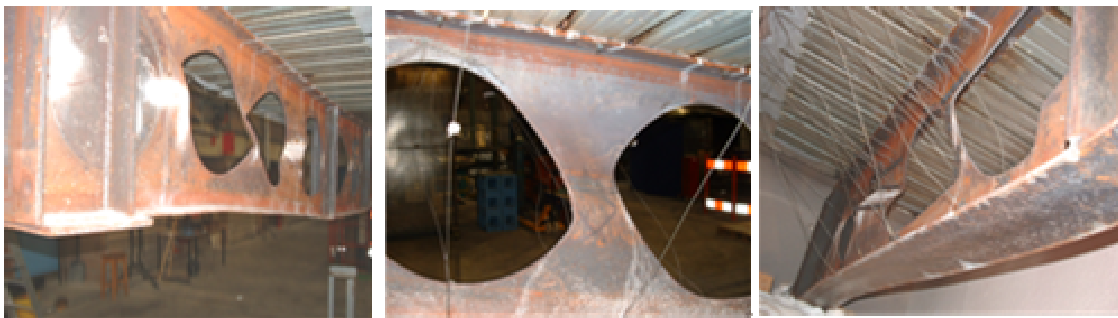
Fig. 9. Web post buckling failure mechanism
