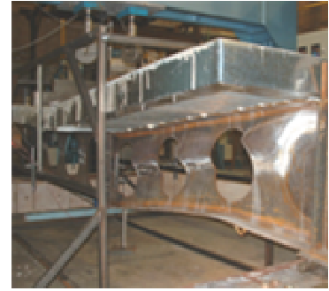
Post web buckling mode failure A1
