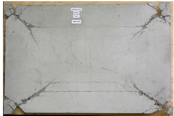
(b) Compressive concrete failure at corners
