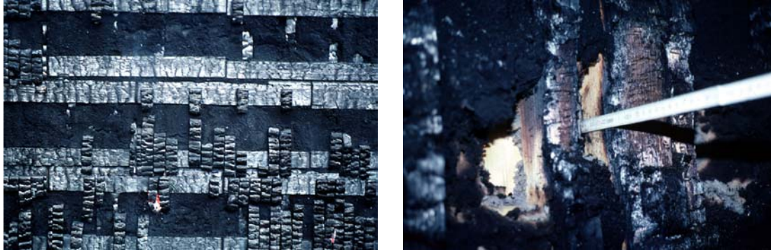
Fig. 9 – Left: wall 1 after the fire test with the fire exposed outer layer completely charred. Right: Detail of wall 3 after the fire test showing a web and a stud partially charred. The isofloc cellulose insulation did not fall into the furnace and protected the wide sides of the webs and studs from charring.
