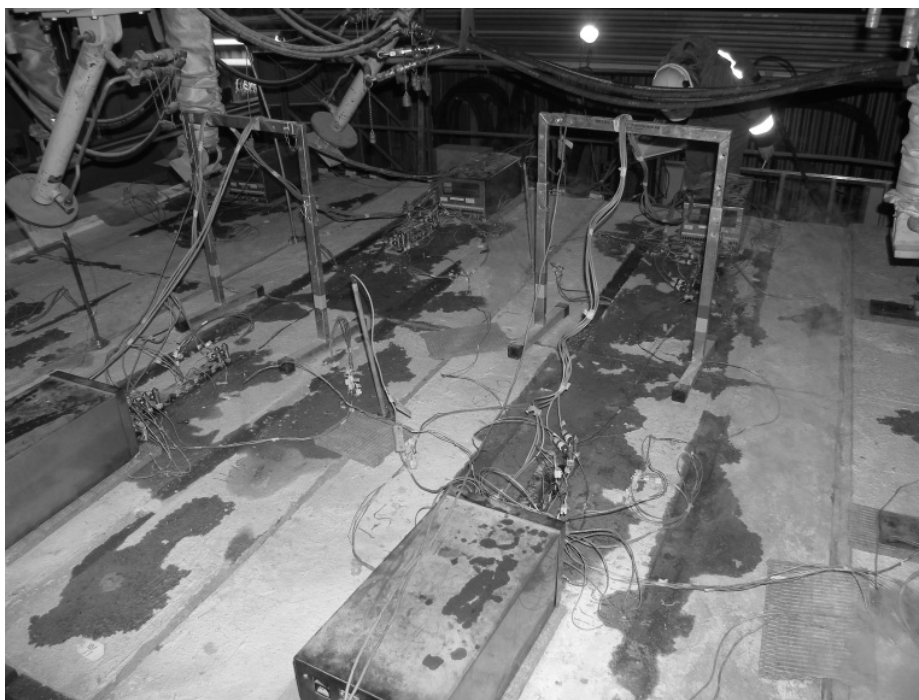
Fig. 1 Liquid water on the non-(fire)-exposed side of 200 mm thick concrete slabs.
