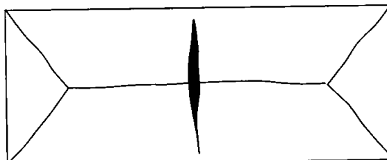
FIGURE 1: Cracking pattern observed in slabs due to tensile membrane action.
