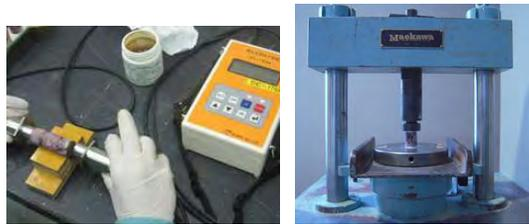
a) UPV test      b) Compressive strength test
