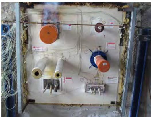
Figure 5. Small scale fire tests assembly (setup 2 - EI90)
