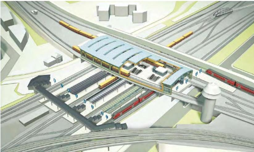
Figure 1. Crossing station in Berlin with overlapping platforms (Source: Deutsche Bahn)
