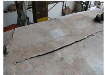
c) Fracture of reinforcement
