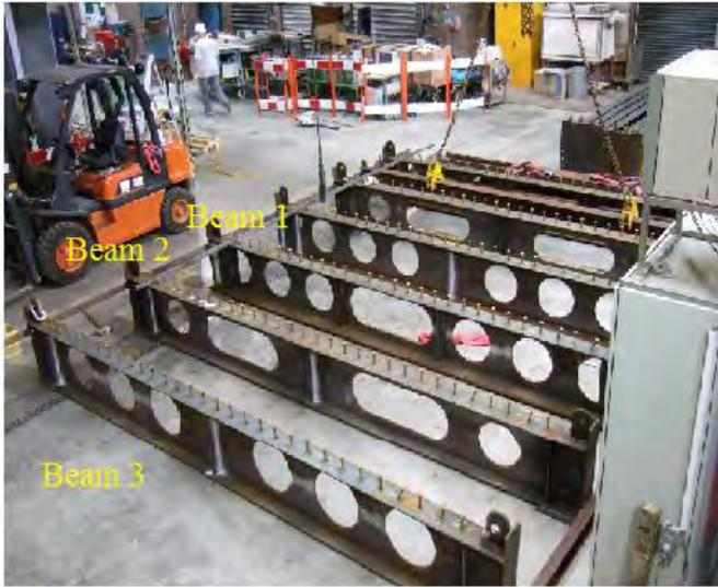
Figure 1: Cellular Beams geometry
